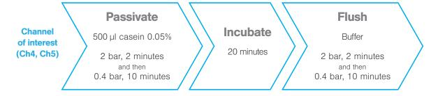
Other channels: same series of steps, but with Experiment buffer only. (2 ml per channel).
